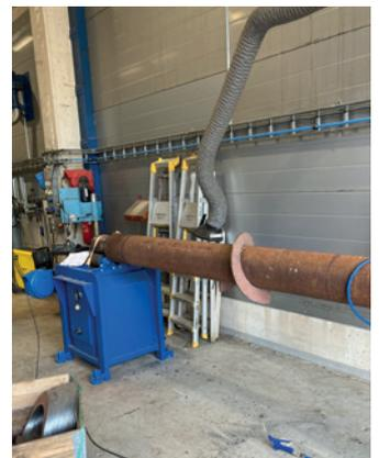
Photo: Screw for discharging cutter shavings produced in the maintenance department with a welding jig developed in-house.
